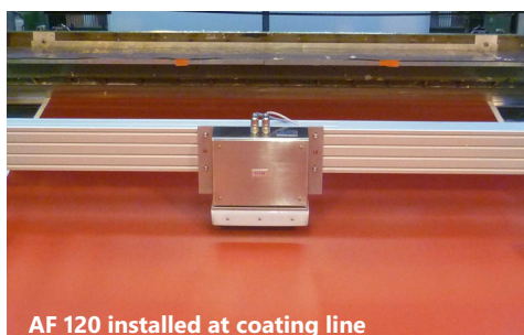
AF 120 installed at coating line
